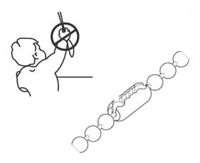
Two breakaway connectors are fitted to the chain of your blind which allows the chain to snap apart under a certain amount of weight pressure. This eliminates the risk of strangulation to young children.
