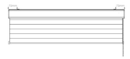
Depending on the width of your blind, you will be provided with a certain number of brackets. For the smallest blind you will receive at least two brackets. These brackets should be mounted approximately 75mm from each end of the blind to ensure an even and stable fit. Any additional brackets you have received should be spaced evenly between these to support the larger width of the blind.
