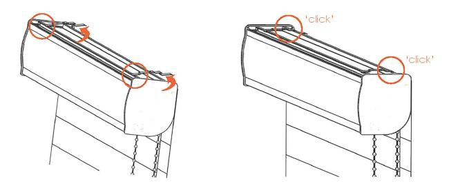
With the cassette tilted away from you (towards the brackets), locate the front lip of the cassette into the bracket and twist into position until it clicks. Your blind is now secured in position.
